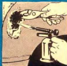
Heated dent is cleaned with steel wool dipped in soldering fluid. Paint is first sanded off. Sheet asbestos protects finish.
