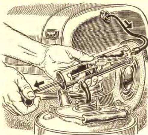
**Spray Gun Siphons Gas.** A siphon for drawing gas from a tank can be made out of an insect spray gun. Take out the plunger and reverse the cup leather. Cut off the spray container, enlarge the hole in the end of the cylinder, and solder in a piece of  $\frac{1}{8}$ " copper tubing. Solder a delivery tube near the other end.
