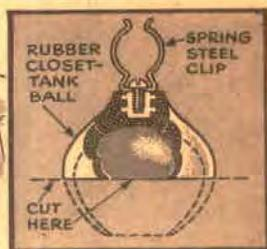
**1 RUBBER VACUUM CUPS** with strength enough to hold light articles on top of your car can be made from discarded flush balls that your plumber may be glad to save for you. There should be no puncture in the upper part. Cut off the balls about  $\frac{1}{2}$ " below the halfway mark and face the edge on a rough emery wheel. Affix a spring clip to each threaded top.
