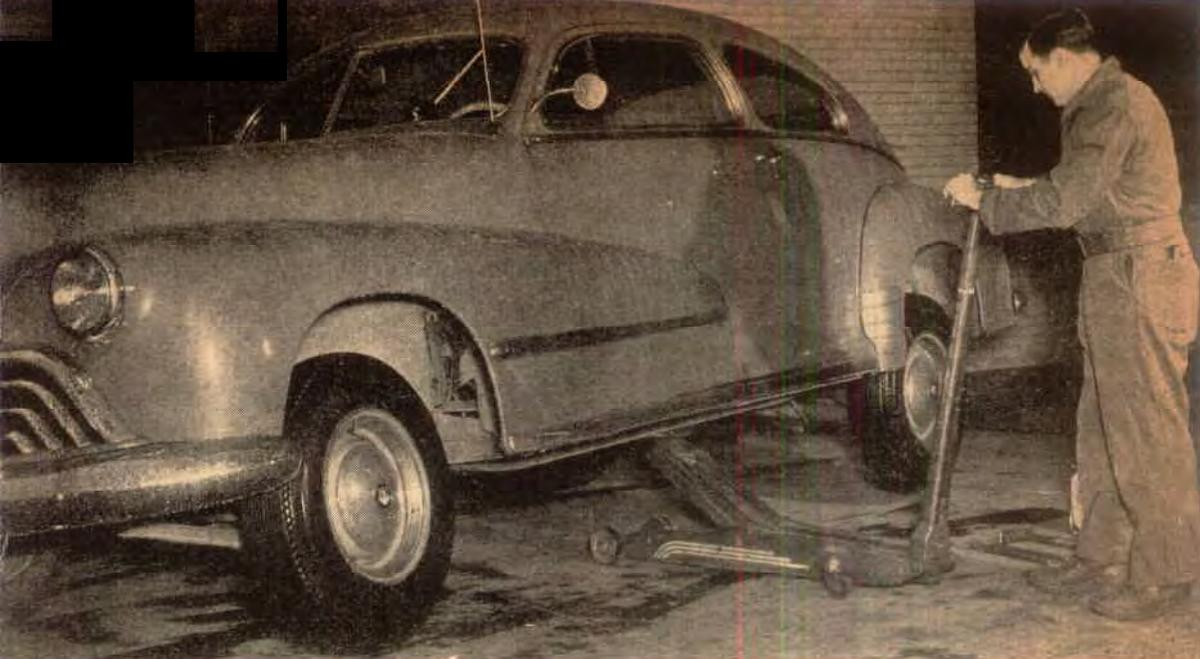
**1. Jack up the car.** That's the first step when tires or tubes are fixed at the General Tire
