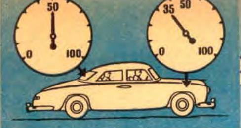
Now you're in overdrive. With pawl engaged, control plate keeps sun gear from rotating. Drive is now from main shaft to pinion cage through splines. This causes the sun gear, transmitting to the outer ring gear, thence to the planet gear, and finally to the output shaft. The sun gear makes only 10 percent as fast as the planet gear. The planet gear, pinion cage makes only .7 revolution on its own axis.
