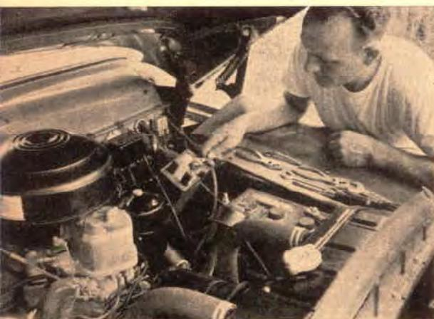
Here's the control box. The two pegs projecting from the end are part of my safety system. Free to move lengthwise through the box, these rest against the gear-shift control rods. The engine can start only if car is in neutral. If a gear is engaged, the bars move, breaking an electrical contact. The box has another job, too, but I'll explain that later. From the box, a wire runs to a powerful solenoid starting switch installed in place of the original one.
