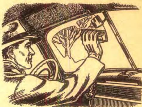
**Eraser Cleans Windshield.** George A. Smith, of Quarryville, Pa., suggests that a clean blackboard eraser is a handy item to carry in your glove compartment. When moisture collects on the inside of the windshield, a few strokes with the eraser will quickly give you unobstructed vision.
