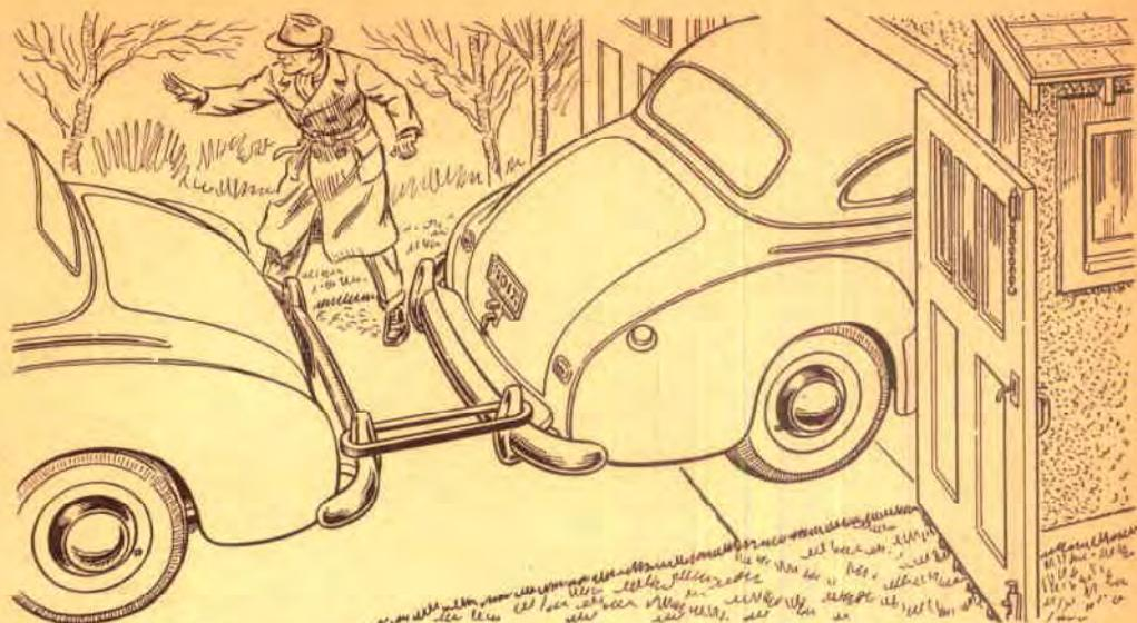
**Fan Belt Gives Tow.** Forrest F. Starr, of Columbus, Ohio, makes a suggestion that may help you out of a tough spot. "My neighbor's car was stuck in soft ground," he writes. "Having no suitable rope or chain, I used an old fan belt. It
