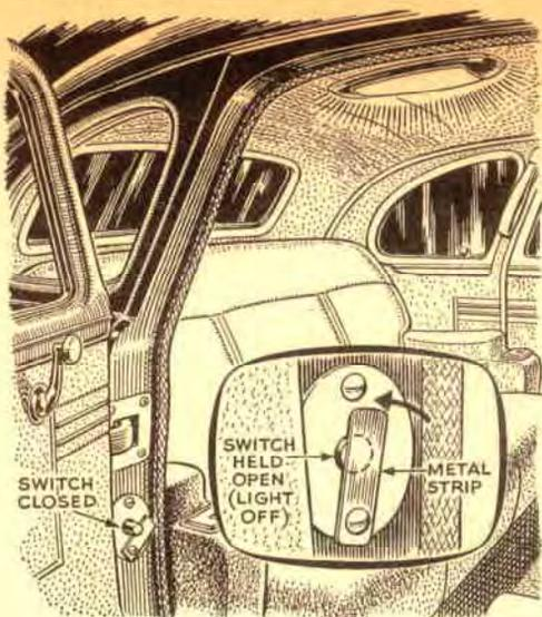
**Door Open, Light Off.** Door-operated dome lights can't ordinarily be shut off if you just want to park with the door open. Wesley E. Charter, of Rockville, Conn., suggests that this can be done with a strip pivoted on one switch screw, preferably the lower one. It takes only a moment then to pivot the strip over the switch button.
