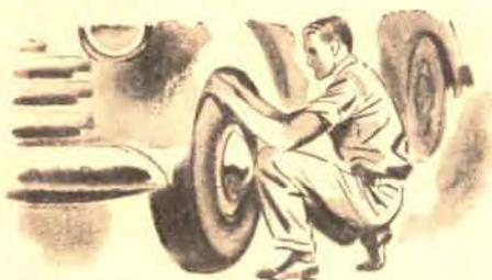
**Are the wheels loose?** Grab a front wheel at the top with both hands and try to move it back and forth in the vertical plane. Can you feel any play, even the slightest? Do you hear a faint sucking noise? The first is a sign of a worn kingpin bushing, the second of a loose wheel bearing. (A damaged wheel bearing makes a clicking sound while the car is in motion. This click becomes more noticeable while you are passing a concrete retaining wall.)
