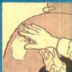
As first step in applying a new finish area is washed with soda to neutralize flux. It is also gone over with pre-priming cleanser.
