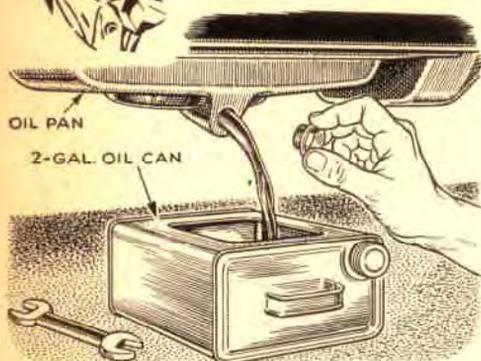
**Oil Drained into Flat Can.** Some new cars are so low that it's awkward to drain the crankcase without a lift. The job calls for a shallow but capacious pan. Victor H. Lamoy, of Upper Jay, N. Y., reports that an empty 2-gal. oil can with a large opening cut in one side gets under easily. Leave a lip around the hole to keep the oil from slopping when you drag out the filled can.
