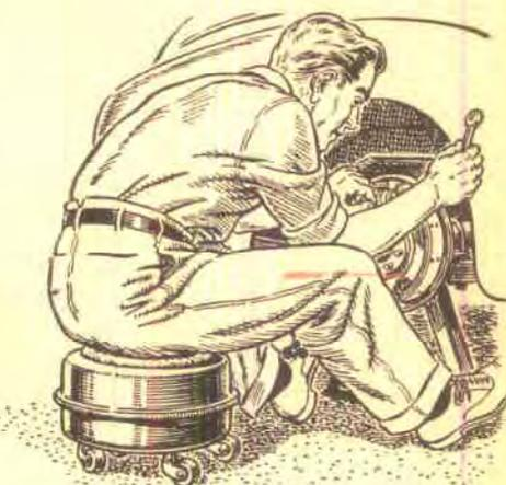
**Stool Built of Brake Drums.** One mechanic made his job easier by welding two discarded brake drums together. Four casters on the bottom and a sheepskin buffing pad on top make it a serviceable rolling stool. It's particularly good for jobs for which you'd ordinarily have to kneel.
