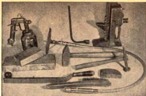
**Few tools are needed** for home fender repairs. The main ones are hammers, a jack, spray gun, vixen file, wire brush, dolly, and wood blocks. A flexible-shaft sander-polisher also is useful.
