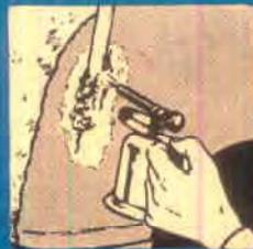
Softened end of solder bar is now jabbed into the dent at several points, leaving enough blobs of solder to fill the dent.
