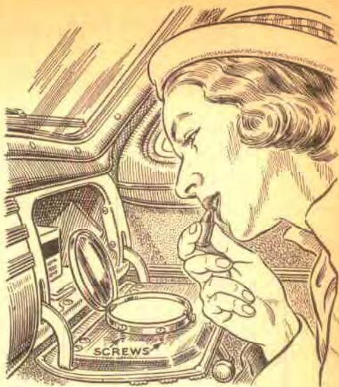
**Mirror Is Always Handy.** Here's the way W. M. Dierks, of Chicago, filled the bill when his wife asked for a convenient mirror for use in the car. Buying a large compact, he mounted it as shown inside the glove-compartment door, drilling holes and attaching it with screws. While not in use, the compact is kept closed.
