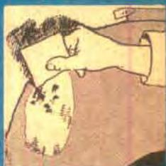
Small blemishes are filled with body putty after priming coat has been smoothed by wet-sanding. Finish in usual manner.
