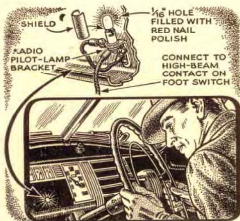
**High-Beam Indicator for Old Cars.** If your car is an older model not fitted with a high-beam headlight indicator, you can quickly remedy the situation. R. L. Parmenter, of Middleboro, Mass., did the job as shown. Ground one of the lamp terminals. Drill a 1/16" hole through the dash ahead of the lamp and fill it with red nail polish. A fiber shield fitted around the lamp keeps light from showing on the floor.
