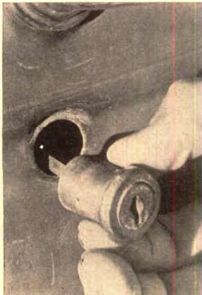
Separate lock units located under the handle are also held in place by one setscrew. When a lock barrel of this type is being replaced, a wire is inserted through the setscrew hole to help guide the square shank into the lock. Be sure to turn the setscrew down flush when it is put back.
