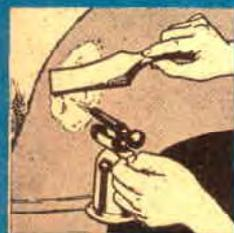
Kept mushy by the flame, the solder is then leveled off to the contour desired. A wood paddle soaked in oil is used for this job.
