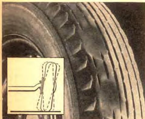
**Wobbly wheels** resulting from such mechanical defects as a bent axle or uneven caster soon make a tire look like this, flat spots being worn in the tread at irregular intervals.
