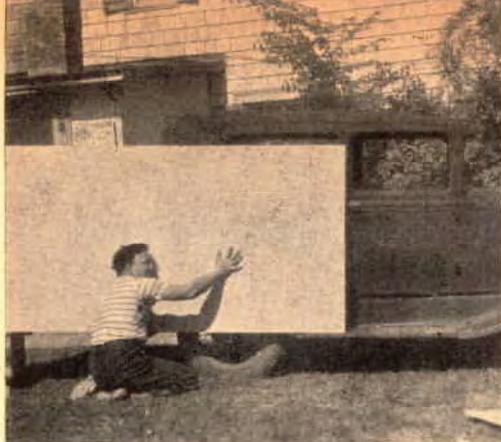
**1** Make patterns of the body panels from fiberboard, using your sketch as a guide. After lining up the pattern sheet, mark it on the inside with a pencil for the fender cutout and for cutting to the lower edge of windows.
