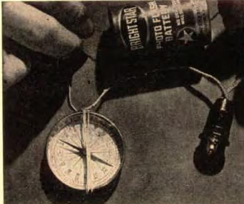
**An ammeter keeps tabs on car battery circuit** by telling whether battery is charging or discharging. You can show in principle how one works. Wind several turns of wire around a pocket compass. Then turn the compass so that needle is aligned with the turns. If you connect a flashlight cell in series with the wire and a
