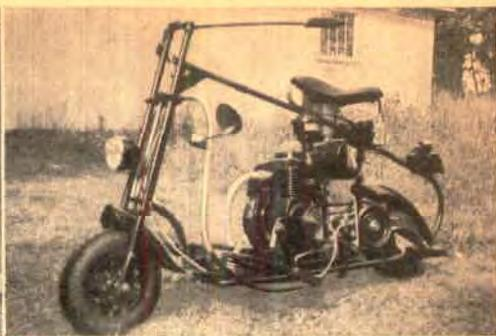
**Scooter Takes Hills Easily.** Employing a reduction of about four to one from motor to driven wheel makes this little scooter an excellent climber. Since it uses a 2.3-hp. engine, it still has enough power to cruise at 35 m.p.h. The Rev. J. Karlton Dewey, who built the machine, used  $\frac{1}{2}$ "
