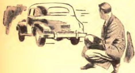
**Do the wheels track?** Rear wheels should follow front ones squarely. You can tell by riding behind the car or watching as it is driven off. Also note whether the wheels wobble, which can be a sign of a bent axle.
