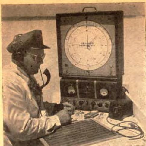
**Electronic stop watch**, calibrated to 1/1,000 of a second, times hot rods during speed runs. Shown with the apparatus is man who designed it, J. Otto Crocker, a San Diego bank technician.
