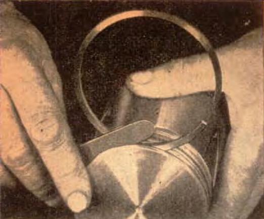
**SIDE CLEARANCE** must be allowed between a new ring and the groove. Measure with a feeler gauge and, if insufficient, lap both sides of the ring on fine emery cloth placed on a flat surface
