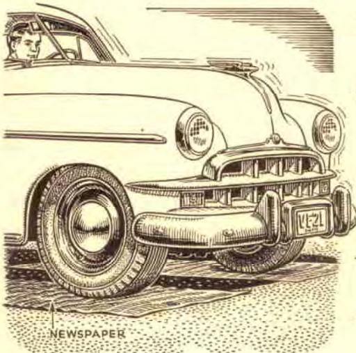
**Paper Tests Brakes.** Not sure which of his front brakes was grabbing, Lewis A. Emswiler, of Etna, Ohio, placed several sheets of newspaper on the garage floor in line with the wheels. Driving on the paper, he applied the brakes. The wheel with the grabbing brake ruffled the paper. It remained smooth under the other.
