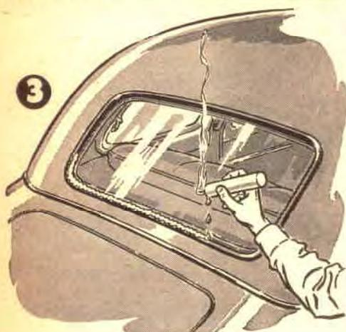
**3. RAIN-LEAKING REAR WINDOWS** and windshields can be plugged with wax dripped from a candle into cracks in the rubber seal. Drip the wax on for several inches on both sides of the breaks. Until the sun melts the wax thoroughly, the leak won't stop completely.—C. D. BASSETT.
