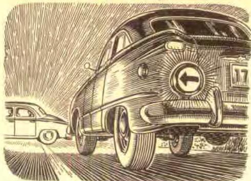
**Light Does Double Duty.** An accessory back-up light—the kind controlled by a separate switch—can be put to extra use as a direction indicator. Using red paint, I painted on the lens a big arrow pointing to the left. Now, when I'm making a left turn or pulling away from the curb, I flick the light on and off a few times. I've used the light for some time now and find it does its new job very nicely. It still gives ample light for backing.—*Ray Smiley, Detroit, Mich.*
