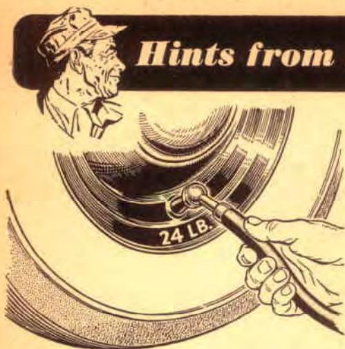
**Prevent Overinflation.** The new low-pressure tires are sometimes overinflated through carelessness. As a reminder to service-station attendants, paint the correct pressure on the rim beside each valve stem with white enamel, or apply waterproof adhesive tape with the figure inked on. You can also buy markers for your caps.
