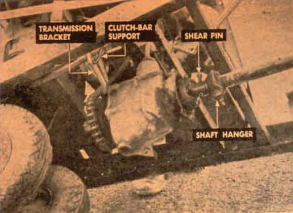
A shear pin protects power train. Universal joint was kept only to make assembly easier. Since rear is unsprung, it could be omitted.
