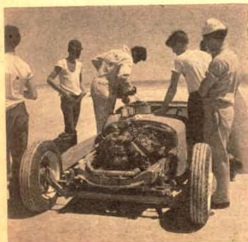
**Radiator is eliminated** to sharpen nose of this model. Instead, it has a 10-gallon water tank behind engine. Car is drained after each run and takes an hour and a half to cool off.
