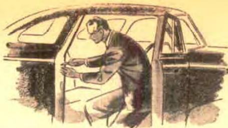
**New paint** may hide a former bright taxi color. Pry up the windshield seal or scratch down to bare metal on an inconspicuous part of the body to see if there's paint of another color. Has lettering on the doors been painted over?
