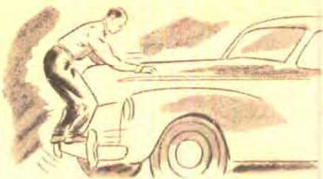
**Test the shocks.** Jounce on the front and rear bumpers. If the car continues to bounce after you jump off, the shocks need repair, or perhaps replacement. (This also tests the bumpers themselves for tightness.)
