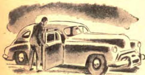
**Sticking doors** suggest that the chassis may have been twisted. Try them all. Also nose the car to the curb at an angle and ease one wheel over the curb. If doors now stick, a loose frame may be allowing the body to twist.
