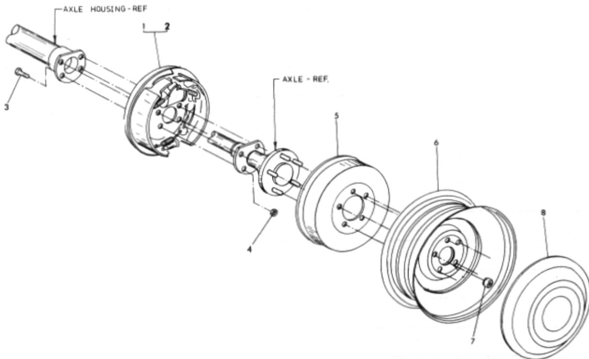
Figure 6-2 Rear Drums, Wheels, Covers Plus Associated Parts
