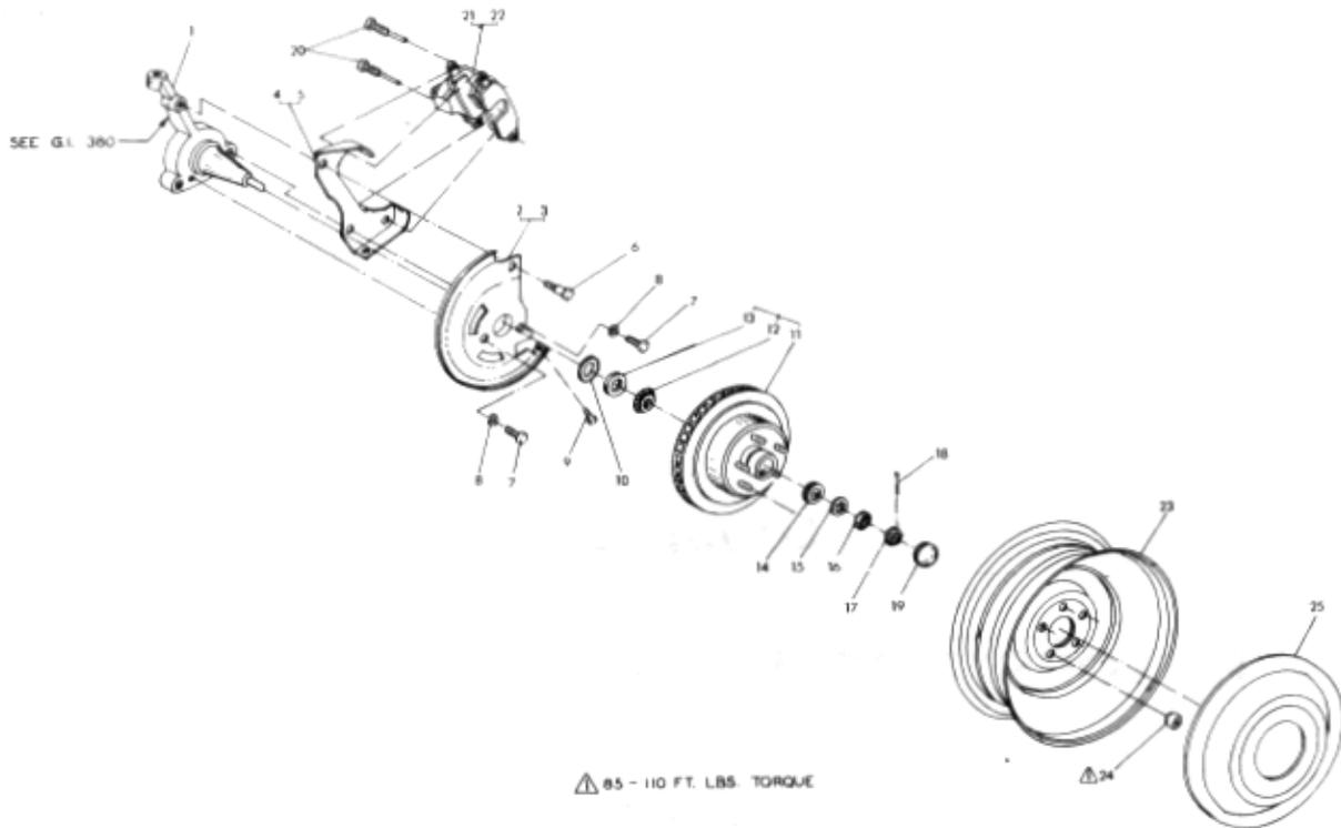
Figure 6-1 Front Hub & Rotors, Wheels, Covers Plus Associated Parts
