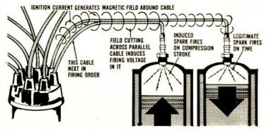
In crossfiring, plugs fire out of time by induced voltage. It causes engine roughness, backfiring, even engine damage. High voltage in a plug cable creates a magnetic field around the cable. Enough voltage may be induced in another cable, close by and parallel, so that both plugs fire.
