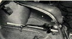
Pontiac also has done something about that noise in the luggage compartment of the family car as the jack, lug wrench, and assorted other tools bounce around with each bump on the road. This year's models have coil-spring tool holders that help stop the clatter of all such accessories.
