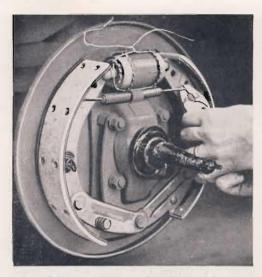
After relining the shoes, replace them in the same order as they were removed. Replace the retracting springs and don't forget to remove wire from cylinder
