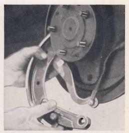
Cable-operated emergency brakes should be checked for free movement of the cables before relined shoes are replaced. Note point of linkage on backing plate
