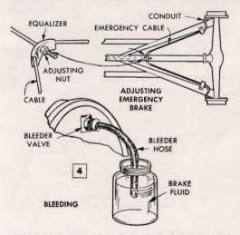
Adjust the emergency brake and check brake-pedal action to see whether air has to be bled from system
