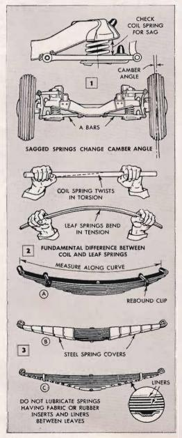
WHEN YOU hit a hole in the pavement or a bump in a side road the shock absorbers snub out the rebound of the car axle. But the springs take the real punishment by preventing the shock from reaching the car frame and body. Even when you're cruising on a smooth highway, the springs soften the ride by constantly flexing to equalize irregularities in the road surface.
