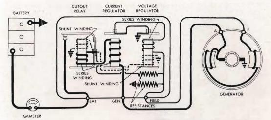
To protect the generator from damage, the cutout relay opens the circuit, preventing a reverse flow of current from the battery to the generator. As shown above, the cutout relay has two windings on the same core
