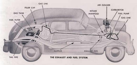
Economy and efficiency in the operation of your car depend largely on the fuel and exhaust system. The typical passenger-car system illustrated indicates several definite and necessary services you should know
