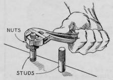
By placing a wrench on one of two nuts locked together, studs can be removed or replaced
