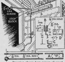
Drawing shows how scraps of wood and iron rod will hold garage doors
