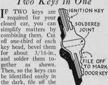
Two keys cut and soldered together to make one key
