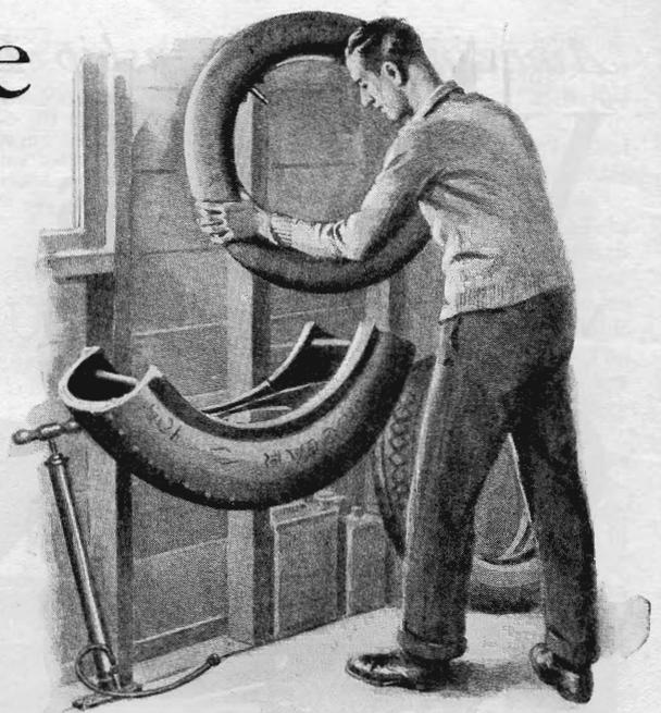
Fig. 4. Section cut from a large truck tire can be used as water container in which to test inner tubes for leaks
