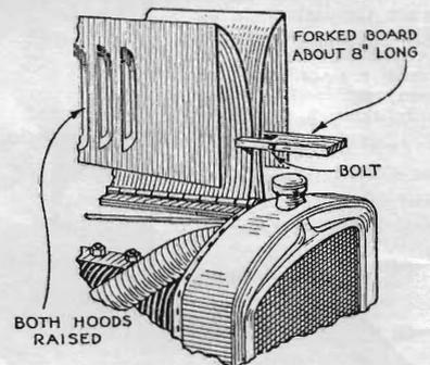
Fig. 5. Forked board, used as in the drawing, makes it possible to raise both sides of hood
