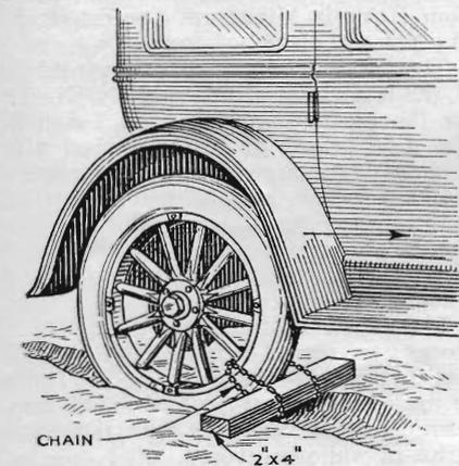
Fig. 1. A piece of two-by-four, chained to wheel, can be used in getting out of mud
