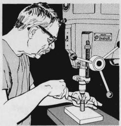
You need three hands to pry the plunger retainer loose from the hydraulic valve-lifter body—unless you use a drill press and a short pushrod to hold the plunger down. This way, you have both hands free for removing or refitting the retainer.
