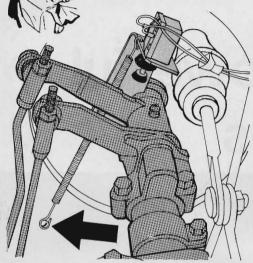
Unreliable backup lights on '56 Fords can be fixed easily by fitting a light spring between the switch bracket and the lower end of the firewall. The spring insures that the reverse bar operates the switch regardless of play in the shift linkage.
