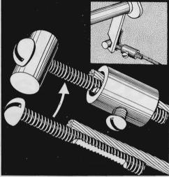
Broken clutch cables on four-speed Corvairs can be repaired by sliding a sleeve over the cable, matching it with a No. 12-24 2" bolt held in the clutch-lever slot by a drilled 3%"-by-34" rod. The bolt threads grip the cable better than a pressed-on tip.
