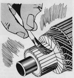
For cleaning brushes and commutators on starters and generators, a good tool is a fiberglass typewriter eraser. Use the eraser end to get down between segments without damaging the mica insulation; reverse the tool to brush out the matter rubbed off.
