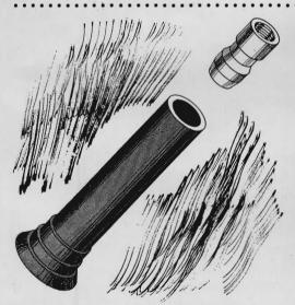
Repair a stripped car-door lock button the easy way by using a screw-on terminal nut or cap from a spark plug as a liner. Drill the button with a  $\frac{7}{32}$  bit (make sure you don't drill through) and press-fit the nut. Screw the lock button back on its rod.
