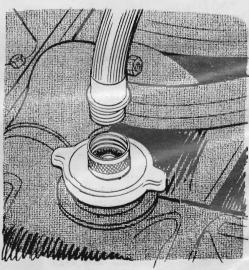
The cooling system of your car can be pressure-flushed with the engine running if you make a special radiator cap Take an old cap, drill a hole in it, weld, braze, or solder a standard brass-hose coupling on top. This prevents splash and gives a powerful flow.
