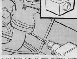
If the large nuts on your manifold studs freeze so tight that even heat fails to loosen them, you can get them loose by drilling a 1/4-inch hole in one side of the hex nut, right through to the stud. This relieves tension enough so that the nut can be unscrewed.
