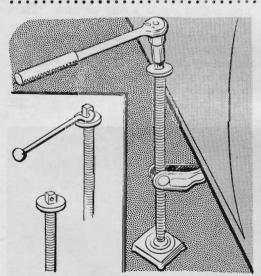
Jack sockets are used in the body sides of most foreign cars, eliminating bumper jacks. On some, the handle makes only half a turn before it must be removed and refitted. A fix: File the top of the jack to fit a \(^3/8\)-inch-square ratchet-wrench adaptor.
