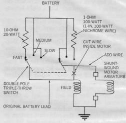
A single-speed wiper can be converted to three speeds. Here's how: The motor must be opened, and a separate lead brought out for one side of the field winding. Switch and resistors are connected (as shown). Nichrome wire is mounted by two small screws.
