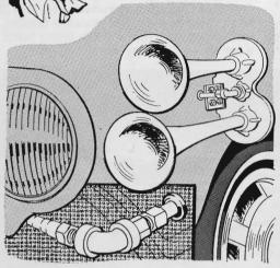
Freon-powered horns are inexpensive, but they require external mounting for maximum sound effect. For best appearance, use two 1/4" threaded pipe elbows with about 14" of 5/16" copper tubing, plus two couplings, one adapter, and four grommets.
