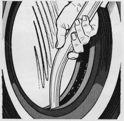
When you're repairing a damaged tire, it's a good idea to get out the vacuum cleaner. Poke the nozzle inside the casing of the tire after dismounting it, and suck out dirt and grit. You'll get a cleaner repair-and less dirt on your garage floor.
