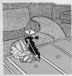
Cut a hole under the back seat in a VW to get better access for clutch adjustment. An opening 2" in diameter will let you reach the threaded end of the clutch cable. Cover the hole with a sheet-metal lid attached with self-tapping screws, as shown above.
