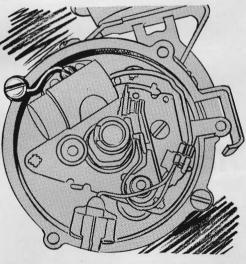
If a Chevy II burns breaker points beyond reason, the cause may be simply excessive resistance from the coil to the distributor. The fix: a short pigtail of small-gauge wire fitted between the condenser base and the distributor plate's retaining screw.
