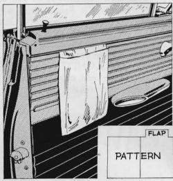
A pocket for odds and ends attached on the inside of a car door is handy. Cut it out of heavy plastic, and heat-seal or cement the edges. Leave a flap at the top that can be slipped underneath the window molding after the screws have been loosened.
