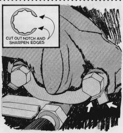
Removing exhaust manifolds of '56-'58 Chevy V-8s can be tricky. Bolts are so placed, it is a job to unclinch locks to get at the bolts. Use a six-point %6" socket, remove a small portion, sharpen edges. When the bolt is turned, the lock will be pushed open.
