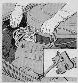
A faulty primary wire on '60 Fords can be replaced without removing the distributor, if you take the wire off the point terminal, tie a piece of cord in the clip hole. Pull primary wire, untie the cord, tie it to new wire, pull it back through the distributor.
