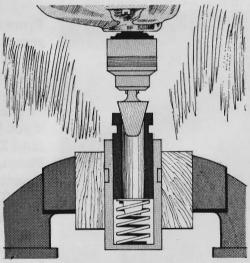
Dismantling a hydraulic valve lifter can be slow when the plunger sticks in the body. Fit a wood plug in the chuck of an electric drill, and insert it in the lifter (mounted in a vise). Press down and start the drill and the rotation will loosen the plunger.
