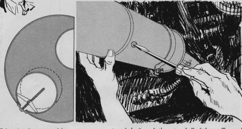
Exhaust noises caused by pressure waves in the gases are regular and normal. If a muffler begins to rattle, however, the cause is usually mechanical failure. Most common defect inside a muffler is a loose baffle tube. It can be fixed without removing the muffler. Drill a ½"
