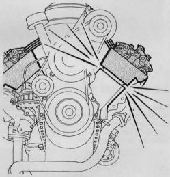
Sticking cylinder heads on V-8s may be broken loose with engine power. Back the head bolts out about %" on one bank of cylinders, keep the plug leads on, and start the engine. The head will be blown loose. Then tighten the loose head and repeat the process on the second bank.
