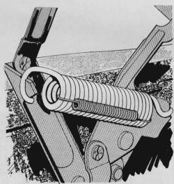
When hood springs weaken so that they cannot hold the hood up, hook a brake-shoe retractor spring to the hood spring. It will add strength to the hood springs. When coating or extra silencing material is added to the hood, the standard springs may be too weak.
