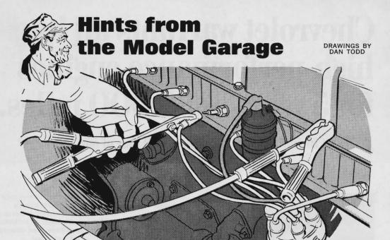
When pulling spark-plug leads off the plugs, one by one, to test the spark or to locate misfiring, you can avoid electrical shocks by clamping one end of a battery jumper cable to a pair of pliers and the other end to a ground connec-
