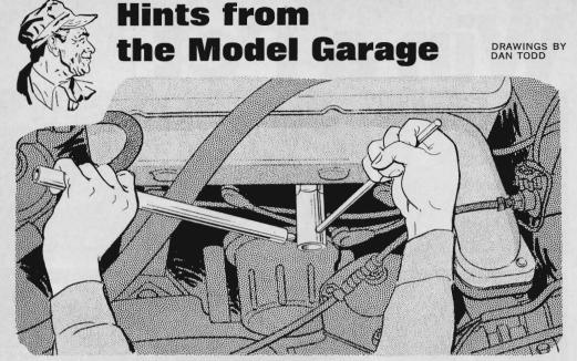
Tight spark plugs in awkward locations that will not come out with an ordinary plug wrench, may be loosened with a long L-shaped handle instead of the short one in an ordinary wrench. The L-shaped handle may be a suitable length of quarter-inch steel rod. The two legs of the
