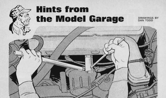
Tight spark plugs in awkward locations that will not come out with an ordinary plug wrench, may be loosened with a long L-shaped handle instead of the short one in an ordinary wrench. The L-shaped handle may be a suitable length of quarter-inch steel rod. The two legs of the
