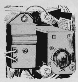
Radio interference in some cases can be traced to improperly grounded two-speed wipers. Here's a simple way to provide proper grounding: Install a 14-gauge stranded wire between the switch plate on the wiper motor and the motor mounting plate.
