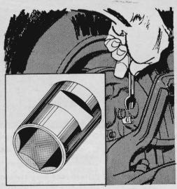
The 1/4" bleed screw on late-model Falcons and Fairlanes is too close to the spindle to let you get a socket wrench and handle in place. The screw is also too small for a normal wrench. Grind two flats on the outside of a 1/4" socket to fit a 7/16" open-end wrench.
