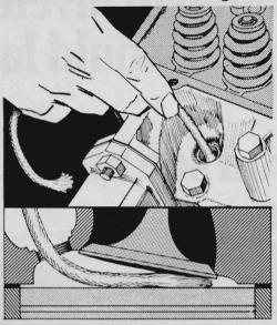
To replace neoprene valve-stem seals you must remove the valve springs. The manual says to use air pressure through the sparkplug hole, with the piston at top dead center, to keep the valve from dropping. If you have no air pressure, drop in a clothesline end.
