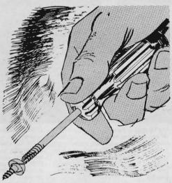
To fit a Phillips screw in a tight place, you often need to mount it on the tip of the screwdriver. To keep it from falling off, fit a small coil spring around the blade and bend the coil out to catch the screwhead. After starting, turn back half a turn to free the spring.
