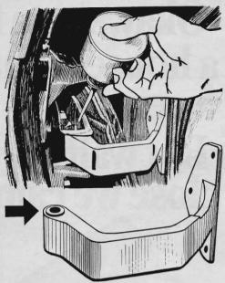
Plastic bushings in the door hinges on Fisher bodies rarely bind. If they do, the best way to free them is with a few drops of transmission oil. This does a quicker job than any lubricating or penetrating oil. Some oils seem to make the bushings bind worse than before.
