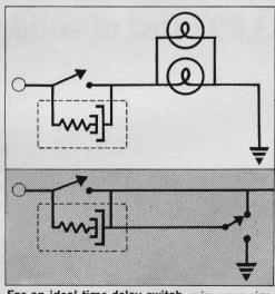
For an ideal time-delay switch, wire your cigarette lighter in series across the headlight switch. Depress the lighter when you leave the car, and unlock your garage or house door aided by your headlights. When the element warms up, the circuit is broken and the lights turn off.
