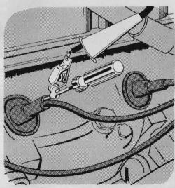
For timing engines, a small plastic-handled screwdriver is a big help. Just force it down alongside the wire and then clip the timing light to the blade of the screwdriver. This simple short cut can save hunting around for a suitable hook-up connection for the light.
