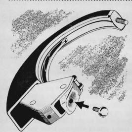
Worn latch-release mechanisms in door handles finally cease to open doors at all. Fix them by drilling a hole in the worn spot on the trip, inserting either a sheet-metal screw or a roundhead bolt to make a higher wearing point. The repair will last for years.
