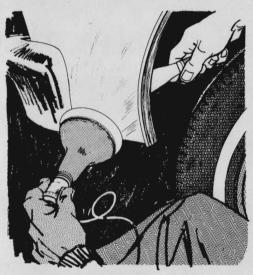
When removing undercoating from inside a fender to reach a nut or bolt, play a heat lamp against the outside. This will warm up the undercoating until it becomes soft and can be removed easily with a putty knife. Do not use a torch, as the hot flame may damage paintwork.
