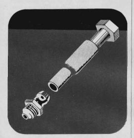
Installing grease fittings in ball joints, steering gear, and universal joints can be made easier if you press the nipple head into one end of a twoinch-long windshield-wiper hose and put a hexhead bolt in the other. Screw the fitting in, pull the hose off, tighten with a wrench.
