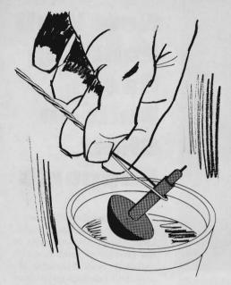
Repairing punctures in tubeless tires in cold weather is hard: The plugs are stiff and difficult to fit. Try this: Bend some wire around the plug and dunk it in hot water for half a minute. This will make the plug more flexible and easier to fit without risk of damage.
