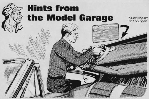
Repairing slits in soft tops is easy with heavyduty iron-on rug tape. Heat settings may vary on different irons-use the minimum heat that will bind the tape. Lower the top to a halfway position and keep the material loosely folded so that when you put the tape on, any sag in the vinyl
