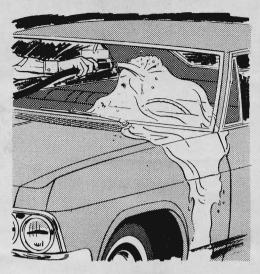
Check out water or air leaks in windshield, window, bolt holes, weatherstripping, by closing all windows and vents, turning on the heater-blower to high, and closing the doors. Run water in a small stream over the suspected area. Bubbles will show up where there are leaks.
