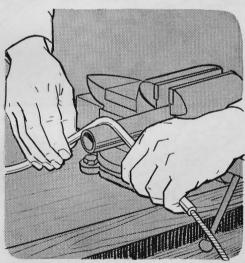
Reshaping a fuel line without crimping or kinking it is easy this way: Put a piece of old speedometer cable inside; then place the line over a pipe and bend it by hand, as above. Pull the cable out past each bend before you make the next, to make removal easier.
