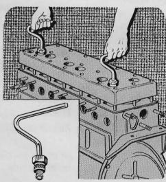
You can make a special tool for lifting sidevalve heads on and off the block by bending lift handles from iron rod. Put the other end through the base of a spark plug. Hammer the end of the rod to keep the plug base from pulling off when you lift the head.
