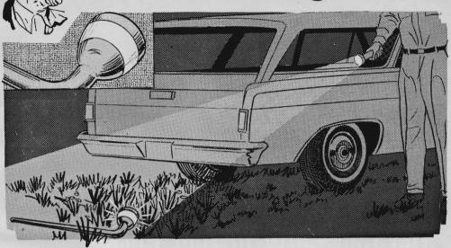
You won't lose a lug wrench or a removable jack base after changing a flat tire on the road at night if you use this simple low-cost precaution. Put a strip of reflecting tape on the tools. When you're done changing the tire, flick your flashlight beam around and
