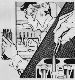
Valve guides can be replaced in pre-'63 Chevy sixes by shrink-fitting them into the head. To hammer them in place could destroy them. Put the new guides in a deep freezer overnight, lift them out with needle-nose pliers, set them in place, and drive them in with a leather mallet.
