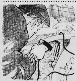
You can check for oil leaks around moving parts with a timing light. Connect as usual, to the battery and to the No. 1 spark plug. The timing light will stop rotation and the motion of the part where you suspect a leak, and allow you to actually see the oil leaking.
