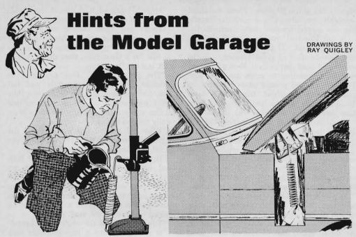
Hood counterpoise springs or brackets on Chevrolets from about 1952-55 can be fixed without special tools. The brace in the fender well is almost inaccessible, and the spring must be extended when fitted. Here's how: Measure the needed spring length for installation. Stretch
