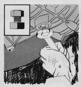
Removing the oil-pan drain plugs from 1960-'62 Volkswagens can be made easy with this simple tool. Weld an 11/16" hex nut to the threaded end of a 1"-long %" hex nut. Insert the smaller nut in the drain-plug recess and unscrew it with a regular open-end wrench.
