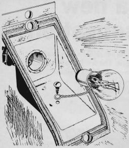
A corroded bulb socket on an older car can lose its ground. Get more life from it by cleaning it and wrapping a piece of bare wire around the brass base of the bulb. Solder the wire in place, and ground the other end of the wire to the lamp housing with a self-tapping screw.
