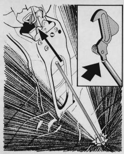
Trunk lockout after body damage on a Corvair can be solved by working through the trunk drain hole. Pull out the rubber plug, cut a hole in the mat, shine a flashlight through the hole, and insert a rod against the retaining clip. An upward push will release the clip.
