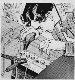
Before recharging a run-down battery in cold weather, check for ice formation in the cells. The surge of electricity from a booster battery can blow up a battery with a frozen cell. If you suspect ice formation, set the car where ice will melt before you hook on the booster cables.
