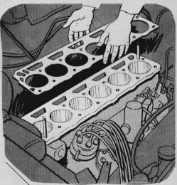
Fitting a cylinder-head gasket on an in-line six is easier if you cut the heads off two bolts long enough to come through the head, saw a slot on top of them, and fit them in diagonally opposed end holes. Drop the pasted gasket on the block, then the head, start a couple of bolts, and withdraw the two line-up studs.
