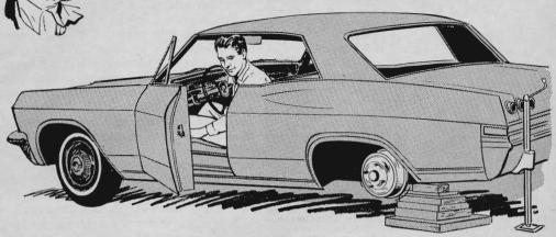
Have trouble removing rear-wheel brake drums from late-model Chevrolets and Pontiacs? Try this: When the drums stick to the axle flange, with the car jacked up and both rear wheels removed, start the engine, engage first gear, and accelerate to the equivalent of 30 or 40 m.p.h. Quickly release accelerator and hit foot brake. Then engage reverse, accelerate, and stop suddenly. Check the drums. If still stuck, do it again. Soon the drums will come loose.
