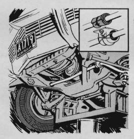
Worn or lost rubber bushings for stabilizer bars can be replaced by scrap from an inner tube rolled around the bar and fitted inside the mounting hole. Cut the rubber so it sticks out at both ends of the bracket. Wrap the whole assembly with a piece of 3/32" GI wire. Use enough rubber to get a tight fit, push into place.
