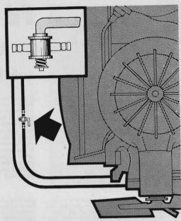
Hard cranking and early firing? Test for end play in the distributor shaft. Connect a timing light to No. 1 plug; disconnect all others. Crank, watching the timing mark. If firing is too early, pull the distributor drive gear and insert spacer washers between the gear and housing.
