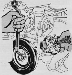
Setting point gap on a Corvair by cranking the engine with the starter and getting the high spot on the cam, is a hit-and-miss deal. For precision, put a %" offset box wrench on the main drive-pulley nut. Moving the wrench turns the cam and enables you to set the gap.
