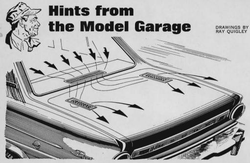
To move hot and stale air out of the car, cut an opening about 1¼" by 12" on the rear shelf and fit an open grille on it. Make sure air can escape through the grille to the trunk. Cut two openings in the trunk-lid sides (as shown) and
