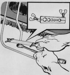
Here's an easy way to remove frozen couplings from the ends of fuel lines, without risk of twisting the tubing open or otherwise damaging the lines. Clamp a flaring tool around the tubing, as close to the coupling as possible, as you unscrew the fitting with a wrench. This works on brake lines with frozen fittings, too.
