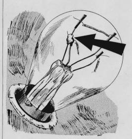
When a brake light won't function and the parking lights come on instead, check the bulb. One filament in a dual-filament bulb can short it internally. A half-melted filament support may fuse to a good filament and switch the current.
