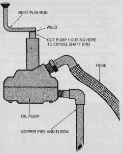
Don't throw away an old oil pump. You can make a handy little pump from it that will have a good many uses; for instance, regreasing a rear axle. The bent pushrod acts as a crank; the pipe is for suction, the hose for delivery.
