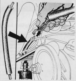
Hooking a dwell meter to the primary side of the coil on a late-model Buick Special is tricky. An easy way is to slide a piece of vacuum wiper hose over a length of 3/16" copper tubing, exposing 1" of tubing on either side. Hook this connector between the terminal and the meter.
