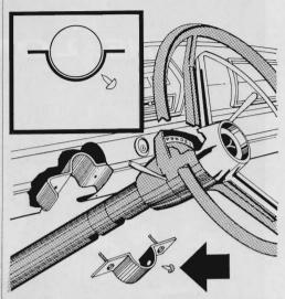
If the transmission indicator light fails on a '66 Plymouth Belvedere, the trouble may be a bad ground connection. Drill a small hole through the support bracket at four o'clock from the wheel (as shown) and insert a ground screw. Make sure the turn-signal wires are out of the way.
