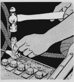
Instead of hammering down on a battery clamp, with the risk of deforming the clamp, the battery post, or both, try this: Place a hollow spark-plug wrench on top of the clamp and tap it gently down. The hollow wrench will drive the clamp onto the post without damage.
