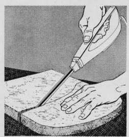
When using foam rubber for trim in a car, you may have trouble finding a suitable cutting tool. Here's a handy tip: About the finest device for cutting foam rubber is a kitchen-type electric knife. It goes through foam rubber fast, leaving a clean cut without shreds.
