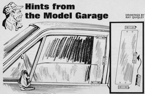
Rain and drafts when a door window is partly open can give you trouble on a '65 Plymouth. This happens because of an inward slant in the glass as it is lowered or raised. To fix it, get a piece of Plexiglas and cut it, as above, following a cardboard pattern. Make four 21/2"-by-3/" angle
