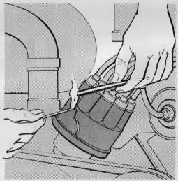
Cracked or burned distributor caps can be repaired with ordinary sealing wax until a replacement is found. Hold the wax so it will drip into the damaged area and melt it with a match or the flame from a cigarette lighter. Make sure the surface of the distributor cap is clean before you apply the wax.
