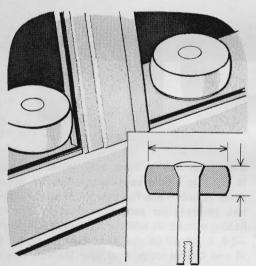
Door-lock buttons give a poor grip? Many do, especially if the locks are hard to operate. One fix: Make a %-inch Micarta ring, countersunk in one surface, to fit the button. Remove the button, fit the ring, and reassemble. Now your fingers can easily grip the button, and the doors can be easily unlocked from inside.
