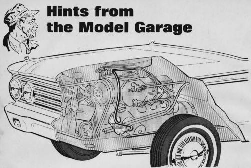
When vapor lock persistently occurs on airconditioned 1961-63 Ford V-8s, first make sure fuel-pump pressure is up to specification, then cut the metal fuel line from the gas tank a few inches from the fuel pump and replace it with
