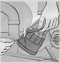
Cracked or burned distributor caps can be repaired with ordinary sealing wax until a re-placement is found. Hold the wax so it will drip into the damaged area and melt it with a match or the flame from a cigarette lighter. Make sure the surface of the distributor cap is clean before you apply the wax.
