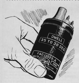
You won't forget the setting for your ignition points any more if you punch the specifications on a piece of "Dymo" tape and stick it on the coil where they can easily be read. Other reminders can be made up and stuck in proper places in the garage as well as in the car.
