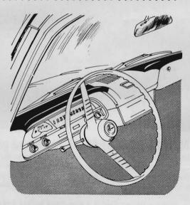
Sunlight reflections of the instrument panel in the windshield bothering you? Here's an effective remedy: Put a coating of flat black enamel on top of the dash. Mark off a symmetrical area with masking tape, and cover it with the reflection-absorbing paint.
