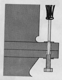
Carburetor bolts inserted from below sometimes cannot be reached with a wrench. But they can be easily loosened or tightened from the top with a screwdriver if the bolt ends have a slot in them. For the final tightening, use a wrench on the screwdriver handle.
