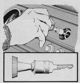
Need a good spot for the spare key? Take the guts out of the cigarette lighter, fill it with epoxy glue and stick the key handle into it. Disconnect the wires to the lighter and remove the back of the socket. The knob now keeps the key handy, but still looks like a lighter — fooling potential thieves but keeping the key handy.
