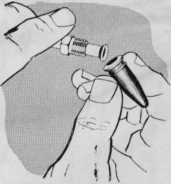
Replacing or overhauling a fuel pump calls for an easy way to stop the fuel flow from the line. The rubber tip from a medicine dropper fits neatly on the end of the fuel line and makes sure no gas is lost. For carburetor repairs, use the rubber tip to keep dirt out of the fuel line.
