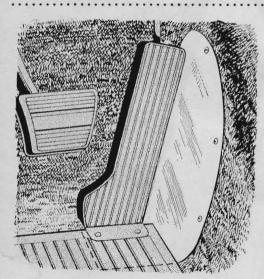
To avoid damage to the carpet around the accelerator, use a small Plexiglas guard. Make a paper pattern, cut the Plexiglas, and sand the edges. Heat the Plexiglas in the oven until it's pliable, form and install it. Extend the guard under the carpet where the heel rests.
