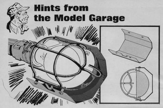
A droplight won't shine in your eyes when you need both hands to work if you make a five-sided shield that fits around the reflector. This will keep the light from rolling over. Start with a small piece of sheet metal and form the four angles by bending it over a sharp-edged piece
