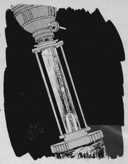
The floats in battery hydrometers and radiator testers are often broken if banged against the side of the tube. To prevent this, keep the instruments filled with water when not in use. Water cushions shock, and your hydrometer or radiator tester will be more safely stored.
