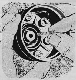
If the carbon piece on top of the distributor shaft breaks, and you don't have a spare, you can improvise one. Take the valve out of the spare tire and use the valve spring in place of the carbon. When you get to a garage for new carbon, put back the valve—and inflate the tire.
