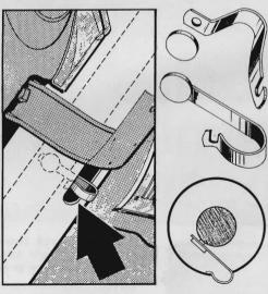
Horns that work intermittently or not at all can be cured by a better ground connection. Fit an old starter brush snugly in the hole at the end of a breaker-arm spring. Insert the spring inside the steering-shaft jacket, near a mounting bracket, where a slot will give access.
