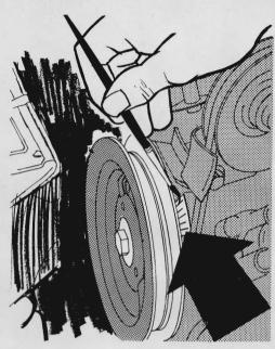
Timing marks (next to the fan-belt pulley) are often hidden under a layer of grease and dirt. To make the marks more visible under the beam of a timing light, try this: Wipe the surface clean and, using luminous paint, fill in the marks with thin stripes of the easy-to-see paint.
