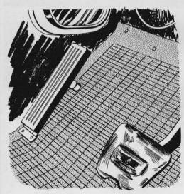
On many cars and trucks, you really have to stretch your foot to reach the dimmer switch. On some autos (especially trucks), you even have to look for it first. To make the switch easier to find, attach an old accelerator pedal to a hinged bracket. Bolt the bracket to the floorboard with the pedal over the switch.
