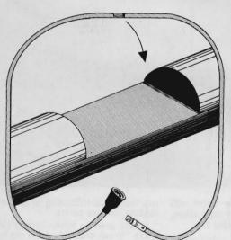
Making a good slip-proof connecting point for a timing light is easy. Hunt up a piece of spark-plug wire (about as long as one plug lead), fit the proper terminals to it, and make a 1/2" cut through the insulation near the middle of the wire. Fit your timing-light clamp in the cut.
