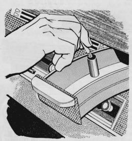
Smoke from cigarette butts in the ashtray is irritating to many drivers. It can be stopped by riveting or soldering part of a lipstick tube to the wall of the ashtray and dropping the butts into the tube. Robbed of oxygen, the fire goes out completely in just a few seconds.
