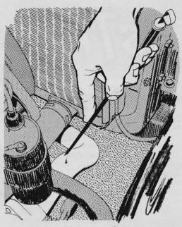
Suspect water leaks? Here's an easy way to check for them: Start the engine and let it warm up. Pull the dipstick and let a few drops of oil drip down on the hot exhaust pipe. If there is sizzling, or bubbles appear, there's water in the oil. If not, there's no leak.
