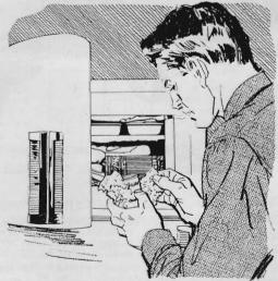
**Test antifreeze strength** this way: Draw off a small amount from the radiator into a can, cover with metal foil, and put it in the freezer (or freezing compartment of your refrigerator). If it does not freeze, the radiator mixture is safe down to approximately zero degrees.
