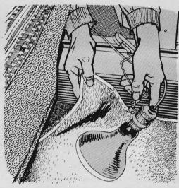
An ordinary heat lamp can make all the difference when you have to remove a carpet or floor mat that is cemented to the car. Hold the lamp so that it shines for a few minutes on each section before you lift it. The infrared heat will soften the cement enough for you to pull the floor covering free without damage.
