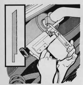
When cutting an old muffler away from an exhaust pipe, there may not be room for a hacksaw. One solution is to make an oversize saber-saw blade: Break a hacksaw in a vise to get a 5" length, grind a shank on it to fit your saber saw. Slow the saw with a speed-control box if you have one in your shop.
