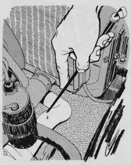
Suspect water leaks? Here's an easy way to check for them: Start the engine and let it warm up. Pull the dipstick and let a few drops of oil drip down on the hot exhaust pipe. If there is sizzling, or bubbles appear, there's water in the oil. If not, there's no leak.
