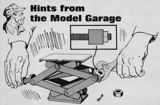
An old automobile jack of the scissors type that is giving trouble often can be easily fixed. Usually, the trouble is caused by the wearing away of the female thread. Where this is the case, back out the male-threaded shaft, reverse
