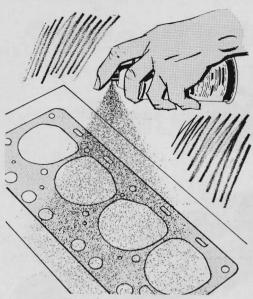
Gaskets can be copied fast and accurately by using an old one as a stencil. Use any leftover aerosol spray paint you have around, and cover the gasket by spraying it straight down. Even the smallest holes will be clear and full size. Remove old gasket, cut and drill.
