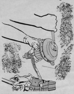
A sticky retainer nut on a generator pulley can be loosened with an oil-filter strap wrench. Place the wrench over the armature and clamp it in a vise. Turning the nut strengthens the grip in the armature, and the nut unscrews easily. To reassemble, reverse the procedure.
