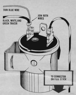
Need a replacement flasher for your VW? The Tung-Sol P-229-D six-volt flasher unit costs about \$1. Join the thin blue wire from the harness to the black, white, and green tracer. This unit flashes immediately, and faster than the one that comes with the VW.
