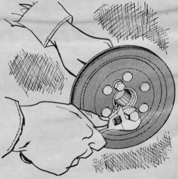
Noisy idling in a Corvair is often a sign that the crankshaft pulley has worked loose from its hub. Fix it by putting two 1/2"-by-3/" standard capscrews with split-type lock washers in the pulley holes. This puts more tension on the pulley and keeps it firmly on the hub.
