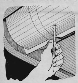
A leaky gas tank can be fixed without draining or removal. Run solder on the threads and under the head of a self-tapping roundhead sheetmetal screw and drive it into the leak site. Tin around the screwhead and solder around it. Avoid red-hot irons or open flame.
