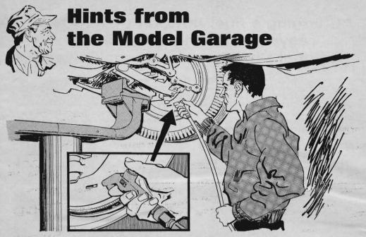
Sometimes brakes will drag or squeal without any signs of mechanical trouble or fluid leaks. If this happens, have the car put on a lift at a service station, leaving all four wheels hanging free to rotate. Aim the air nozzle of the station's air hose into the brake-adjustment slot
