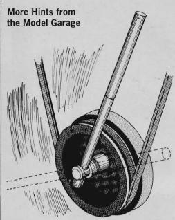
To turn an engine to an exact point, the best way is to mount a socket and sliding T handle on the bolt that fastens belt pulley to crankshaft. Use a long handle to get lots of leverage for large-displacement engines. The handle makes it easy to work without hitting connections.
