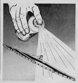
You can use color-matched spray to eliminate glare from chrome-plated wiper arms. Pull the wipers off the hubs, remove rubber, sandpaper arms and blades, and clean with solvent. You won't need a primer if you're careful. Spray according to instructions, let dry, and reassemble.
