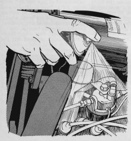
A quick cure for vapor lock in steaming weather (especially for motorists taxing their engines with trailers) is to buy an aerosol can of Freon gas-the type used on self-powered spray guns. Just spray the chilling Freon on the fuel line to the pump, on the pump, and on the carburetor.
