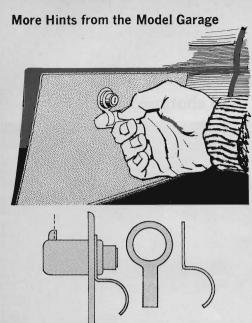
Some glove compartments need a fingernail or a knife to open them when they won't yield to the button. Get rid of the problem by removing the lock and inserting a clip behind the lock shoulder. If you wish, secure the clip with screws, but the lock itself will hold it.
