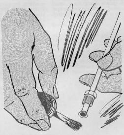
To simplify connecting steel fuel lines with flare fittings to carburetors or fuel pumps, put a film of Permatex #3 or similar compound on the flare's sealing surface. Allow to dry before making connection. Also apply thread lubricant to the flare-nut threads and tubing.
