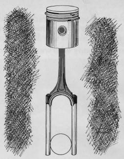
Two short pieces of air hose can help you avoid an exasperating experience in installing pistons and connecting rods in an engine-especially a V-8. Slip the hose on the rod cap bolts to hold the insert in place, and guide the connecting rod onto the crankshaft.
